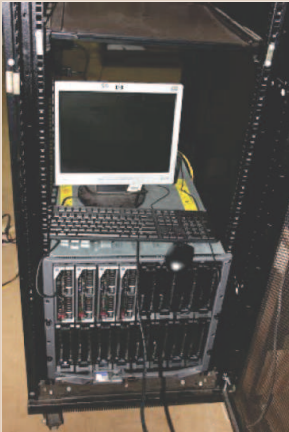
96 core blade server HPC (# of cores in this server is extendable upto 256)
